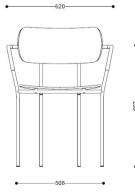
MEASUREMENT - L X W X H MM Sitting height: 47 cm Seat diameter: Ø 48 cm Frame width: 61 cm Frame depth: 41 cm Chair height: 80 cm
