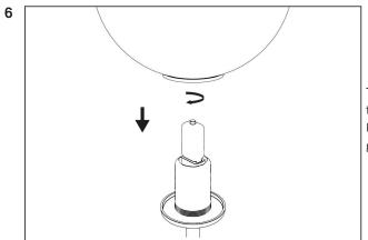
Take the glass globe and carefully place it over the light bulb. Fixate it by turning the glass globe clockwise.
