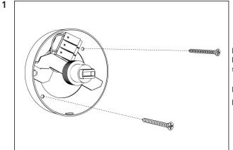
Mount the back part of the lamp to the wall or ceiling with screws.
