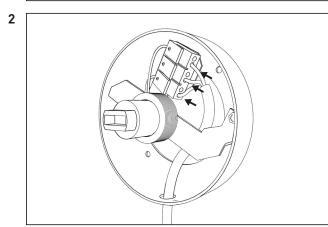
Lead the power cable in through either the bottom or the back of the ceiling plate
