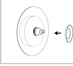
Carefully place the small metal plate over the socket.
