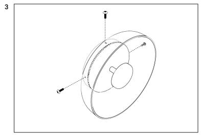
Secure the light fixture with the 3 screws.
