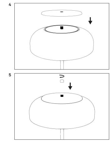
Carefully place the metal plate on top of the glass shade.
