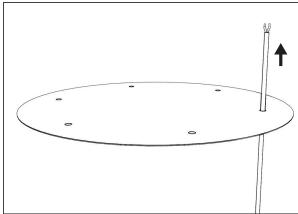
Lead the cables through the cover plate.
