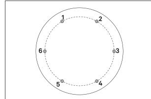
Arrange the cables by numerical order if you want to make an arranged formation
