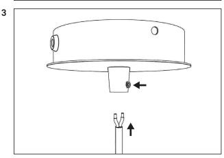
Lead the fabric cable in through the cable relief at the bottom of the ceiling plate.
