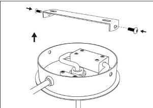
1. Lead the fabric cable into the cable connector.
